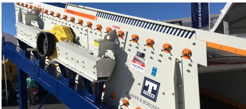
Locknuts installed on shaker table
